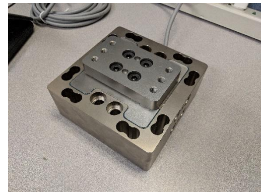
3-axis loadcell
